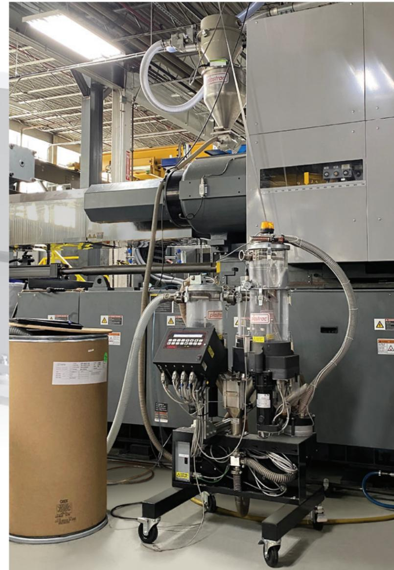
Critical to ColorStream is a regenerative blower that delivers clean transport air, up to 4,000 feet per minute, via a plastic hose having a 1 or 1.25 inch diameter. It keeps transported granules entrained in the air stream without requiring a much larger, power-consuming blower. There are no contacting parts requiring lubrication. The blower is engineered to run continuously for years.
